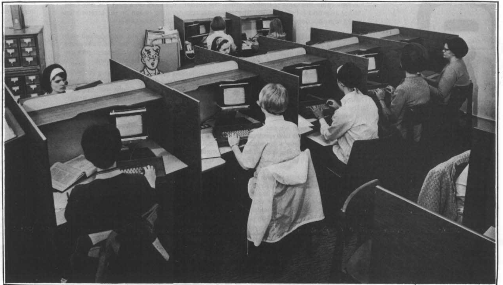
The present PLATO III system consists of a Control Data Corporation 1604 computer and 70 graphic-pictorial terminals 20 of which can operate at one time.
